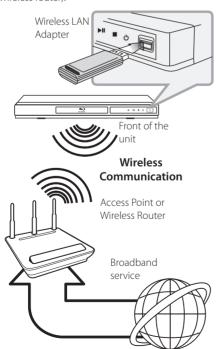
Refer to the setup instructions supplied with your access point or wireless router for detailed connection steps and network settings.
